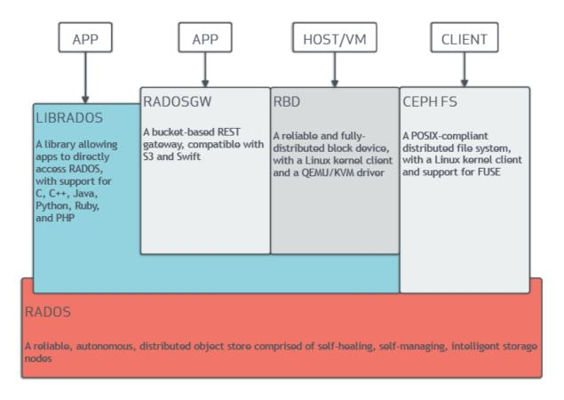
Figure 2: Ceph architecture (from http://docs.ceph.com)
