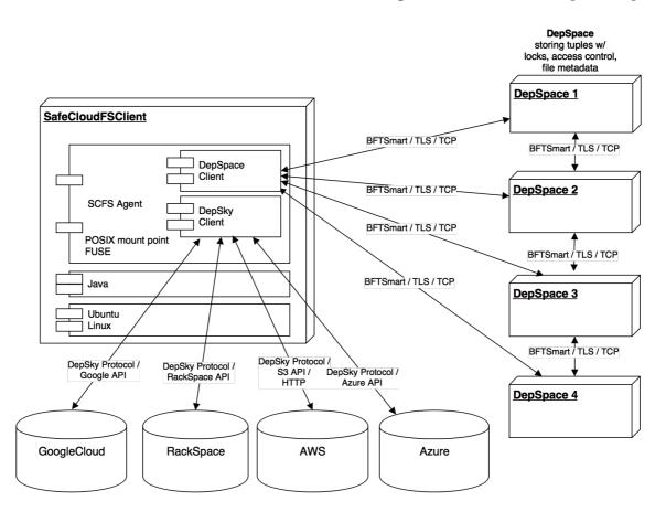
Figure 1: SCFS architecture (image provided by IN-ID)
