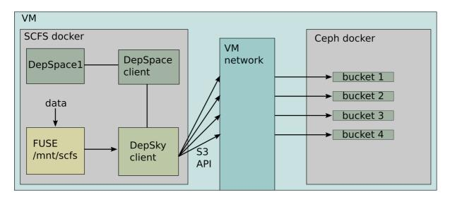
The SCFS + Ceph prototype setup is shown in Fig. 3.
