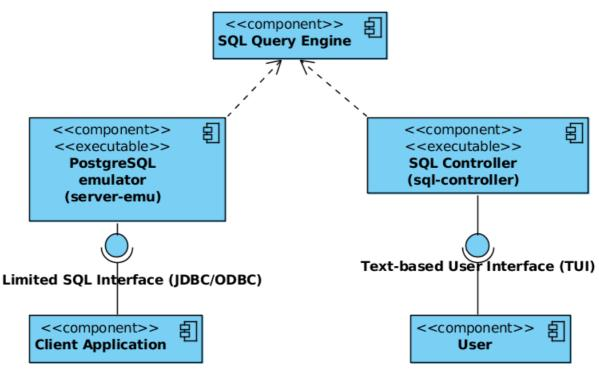
Figure 4: A closer view of Solution 3 frontend architecture deployment
