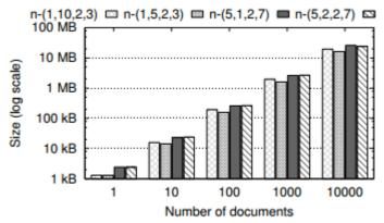
Figure 7 Metadata storage overhead with an increasing number of documents in the archive with different STeP configurations.
